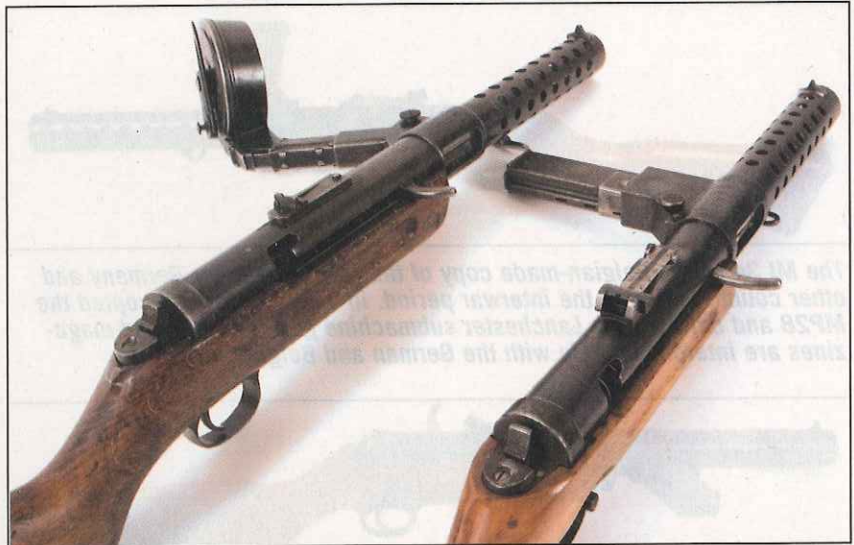
A Bergmann MP18.1 and a Bergmann MP28 (MI 34) side-by-side, illustrating their three main differences: the magazines, the rear sights and the auto/semi selector found above the trigger group on the MP28.
