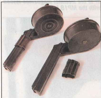
Two trommel magazines showing the feed collar needed to keep the magazine from protruding into the feed ramp of the receiver. It was a simple slide-on, slide-off affair.
