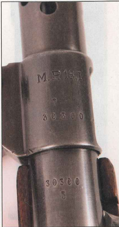
Receiver markings on an MP18.1 are simple and direct: MP18, 1/military acceptance mark/serial number.
