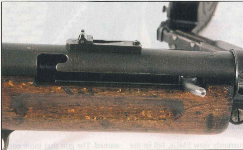
The tube-like receiver of the MP18.1 illustrates the rear notch that served as the safety and the simple L-shaped leaf sight that had apertures for 100 and 200 meters.
