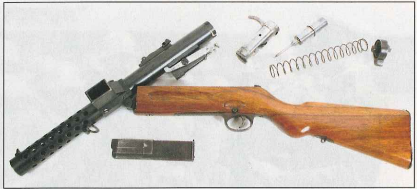
Both the MP28 and the MI 34 have only 65 parts, and breakdown is quite simple, making it easy to clean and repair. It is a standard blowback system with a heavy bolt that kept the cyclic rate to 600 rounds per minute.
