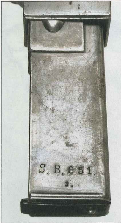
Unit markings found on the reverse of the C.G. Haenel magazine. Bergmann magazines are interchangeable with those later manufactured for the British STEN and Lanchester submachine guns.
